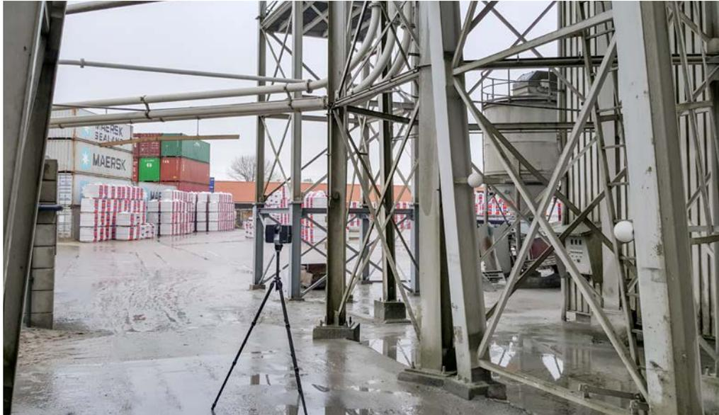
Rapid on-site scanning service with FARO Focus Laser Scanner to create 3D models
