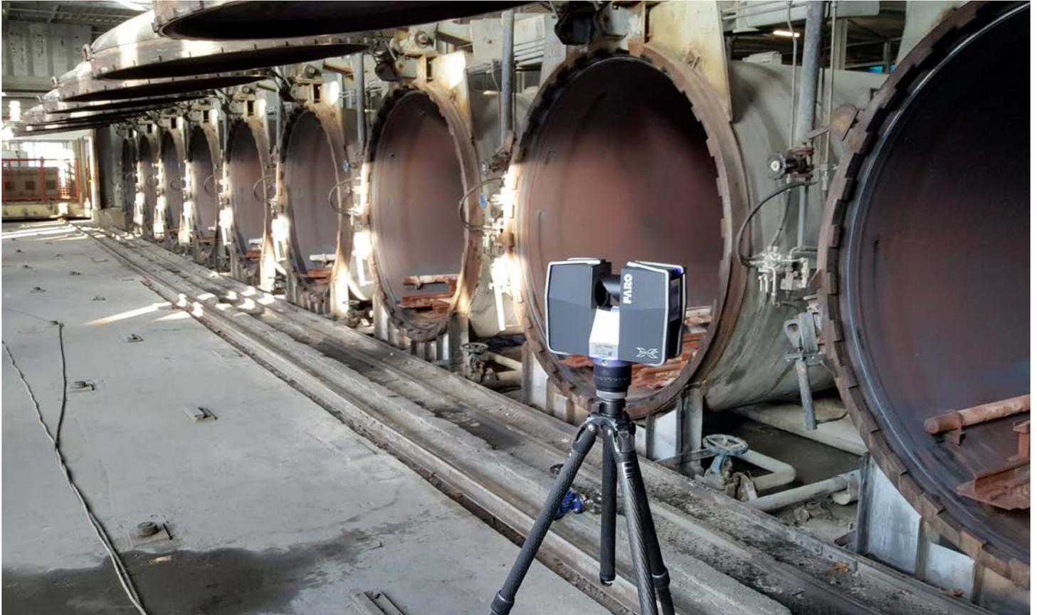
Scanning with FARO Focus Laser Scanner to receive full and highly accurate point clouds and 3D models
